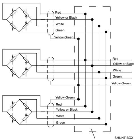
In systems that use several cells, the parallel connection automatically sums the loads on each individual cell.
