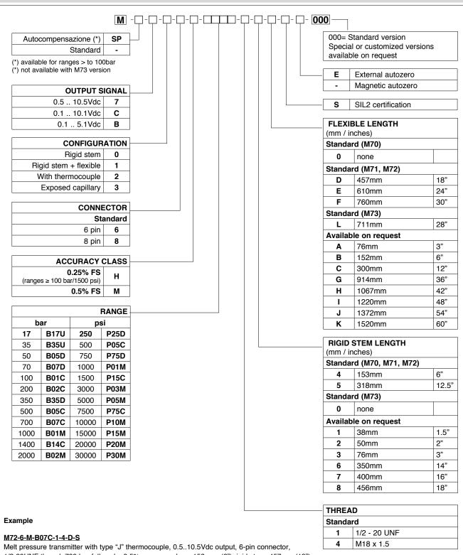
Melt pressure transmitter with type "J" thermocouple, 0.5..10.5Vdc output, 6-pin connector, 1/2-20UNF thread, 700 bar full scale, 0,5% accuracy class, 153 mm (6") rigid stem, 457mm (18") flexible capillary, SIL2 certification.
