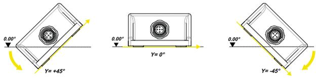
SINGLE AXIS INCLINOMETER ( $\pm 180^\circ$ ) – Z AXIS
